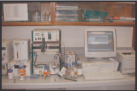
Equipment employed in high-performance liquid chromatography (HPLC) assay of antifungal agents.
