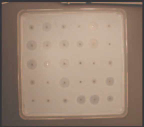
Agar plate demonstrating zones of inhibition obtained by diffusion of antifungal agents during bioassay.
